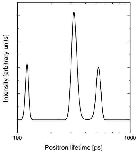
**Fig. 3.** Result of a maximum entropy of lifetime (MELT) analysis of the positron lifetimes of plastically deformed Czochralski-grown silicon (Hübner et al. 1997b). The sample is the same as in Fig. 2 (3.5 % deformation at 775 °C). The peaks obtained correspond well to the discrete lifetimes from the decomposition of the spectrum in Fig. 2,  $\tau_1 = 120$  ps,  $\tau_2 = 320$  ps, and  $\tau_3 = 520$  ps.
