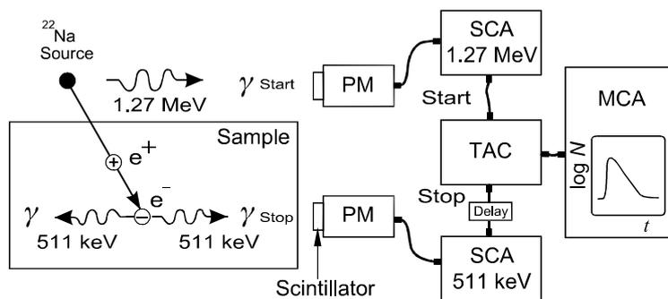
**Fig. 1.** Scheme of the positron lifetime experiment in fast–fast coincidence. The lifetime is measured as the time difference between the appearance of the start and stop  $\gamma$ -quanta (PM—photomultiplier, SCA—single-channel analyzer). The amplitude of the time-to-amplitude converter (TAC) analog output pulse is proportional to this time difference. The whole lifetime spectrum  $N(t)$  is stored in a multi-channel analyzer (MCA).
