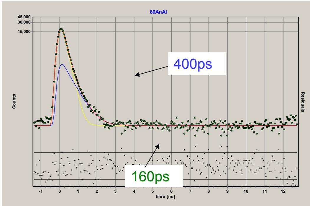
➤ The lifetime spectrum is a convolution of instrumental resolution, source lifetime and the sample lifetime.
