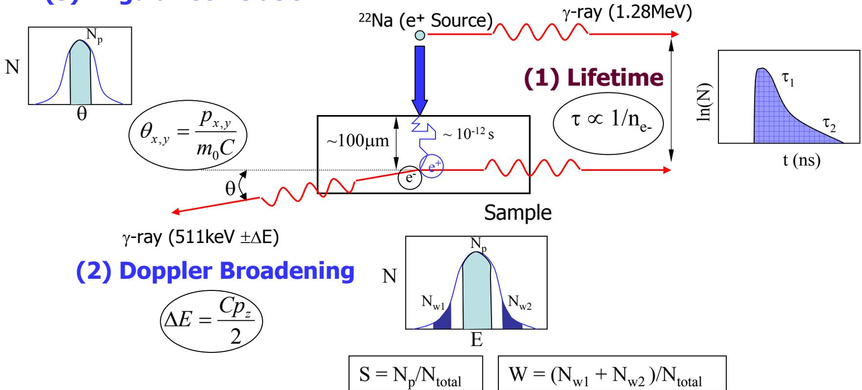
Positron Annihilation Spectroscopy consists of three techniques viz., (1) Positron lifetime (2) Doppler Broadening and (3) Angular Correlation of annihilation radiation.
